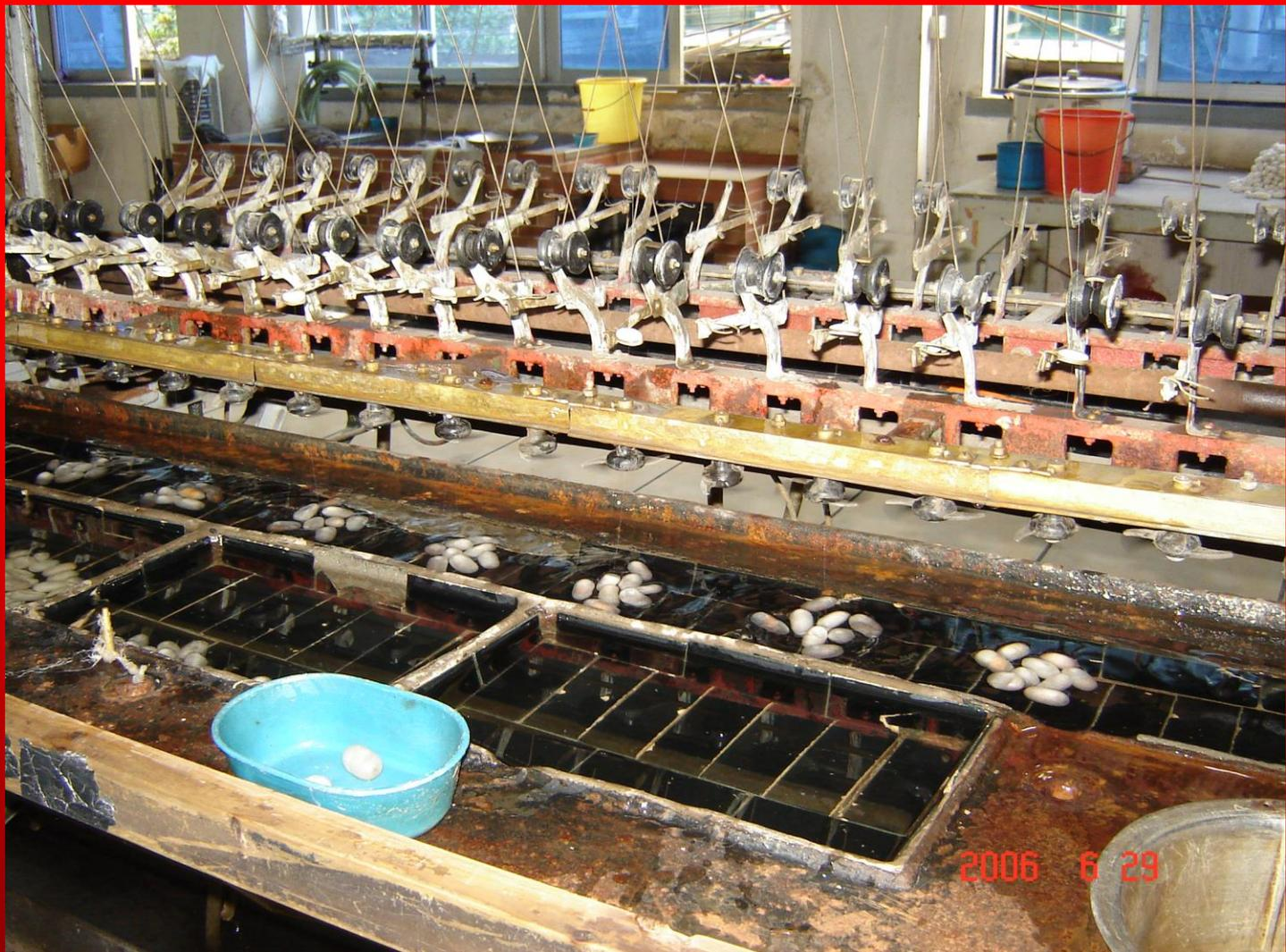
The cocoons lie in water. Then the fine thread is pulled from them and run through the loom above.
