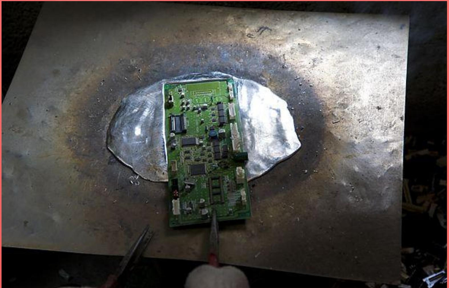
The ewaste is mined for the lead, gold, copper and other metals that are found in the circuit boards, wiring, chips and other parts of electronic devices. In this photo, a worker heats a computer board on a steel surface to remove the computer chips soldered into it.
